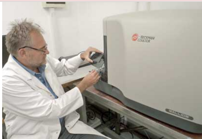
Citometru de flux - Beckman Coulter
