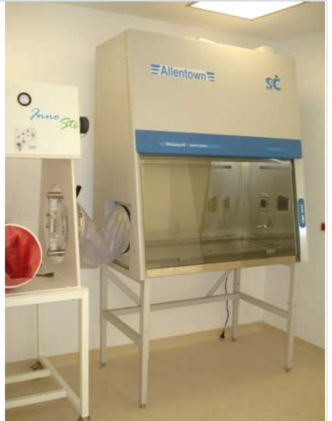
Hota biologica de securitate si transfer de animale – ALLENTOWN, Izolator de transfer mobil 2 manusi - EuroBioConcept
